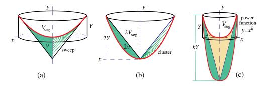
Figure 20. Volume of a paraboloidal segment.
