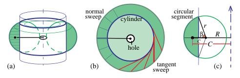
Figure 14. Calculating the volume of a swept solid using Pappus' theorem.
