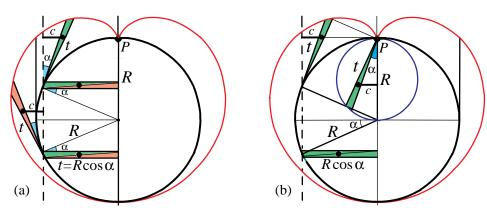
Figure 41. Diagram showing that punctured apple has same volume as the sphere.
