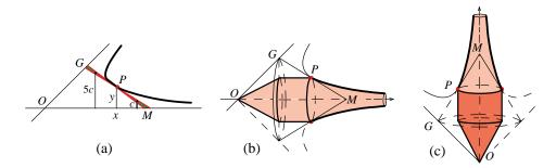
Figure 39. (a) Centroidal distance to upper tangent sweep is 5 times that to the lower tangent sweep. (b) and (c) Hyperboloid of revolution and attached pedestal of equal volume.
