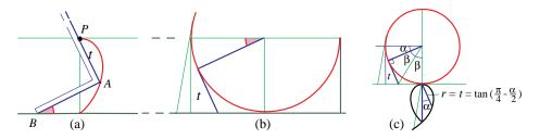
Figure 34. (a) Newton's description of strophoid. (b) Tangent sweep to a unit circle used to describe strophoid. (c) Polar equation describing strophoid.
