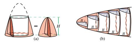
Figure 5. (a) Paraboloidal bracelet has the volume of the solid tangent cluster. (b) Family of paraboloidal bracelets of equal height and equal volume.
